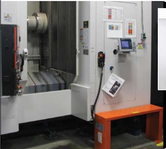
On the outside, the most conspicuous addition to these otherwise “standard” machines is the gaging system’s control and readout unit mounted to the right of the operator’s door on the side of the machine. The inset shows a close-up of the unit.
