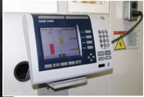
On the outside, the most conspicuous addition to these otherwise “standard” machines is the gaging system’s control and readout unit mounted to the right of the operator’s door on the side of the machine. The inset shows a close-up of the unit.
